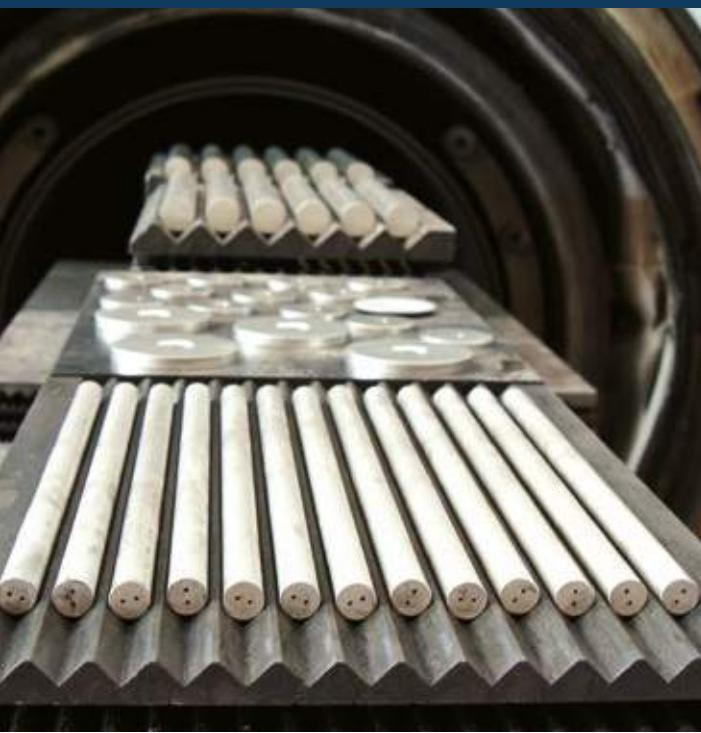
**Coolant rods** - central coolant hole
